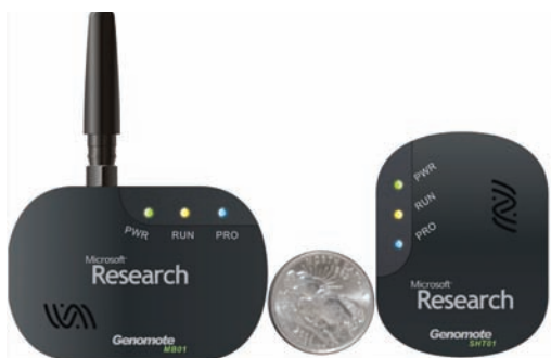
Figure 4: MSR Genomotes with the relative size of a U.S. quarter; master mote (left) and slave sensor (right).
